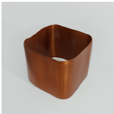
(a) 3D model of a single ISTTOK magnetic probe coil.
